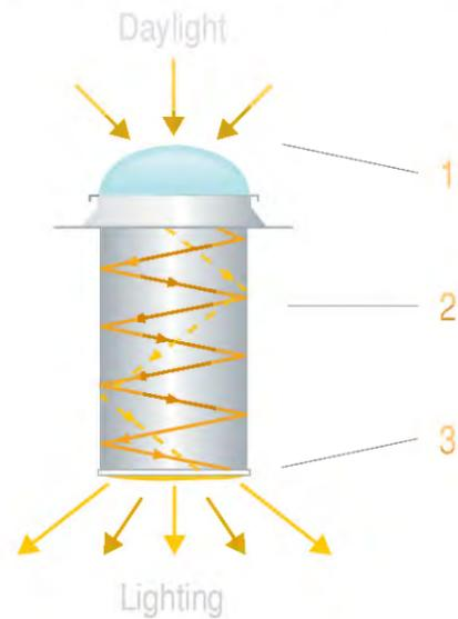
1 Special acrylic dome placed on the roof, passes the daylight on reflecting pipe.
